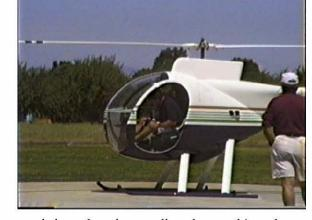
This entry level turbine rotorcraft was designed as a time builder for the rotorcraft student and its 600 lb light empty weight and 500 lb useful load make it the worlds most cost effective rotorcraft time builder.
